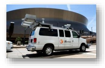
The condition of the roadways was captured via the Road Tester 3000, which was equipped with lasers, inertial GPS and high-definition digital imagery to simultaneously collect the pavement profile, rutting and roadway geometrics. The results of the assessment were used to determine the pavement surface distress and identify where all such pavement conditions exist.
