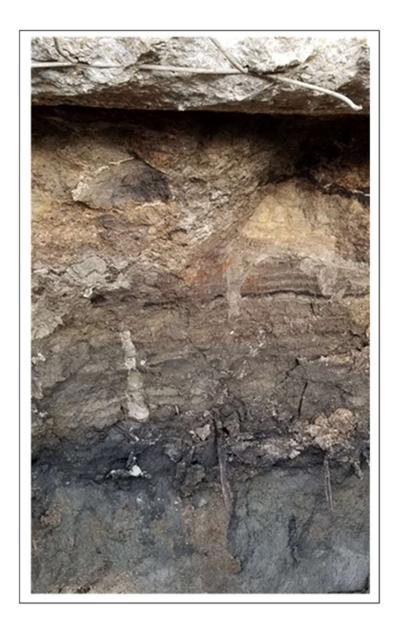
Figure 2. Bluish gray (Gley 2 5B 5/1) sand observed (bottom of photo under dark lens) in water line trench on Wales Street between Exeter and Martin streets. Little Woods Group A, RR100.
