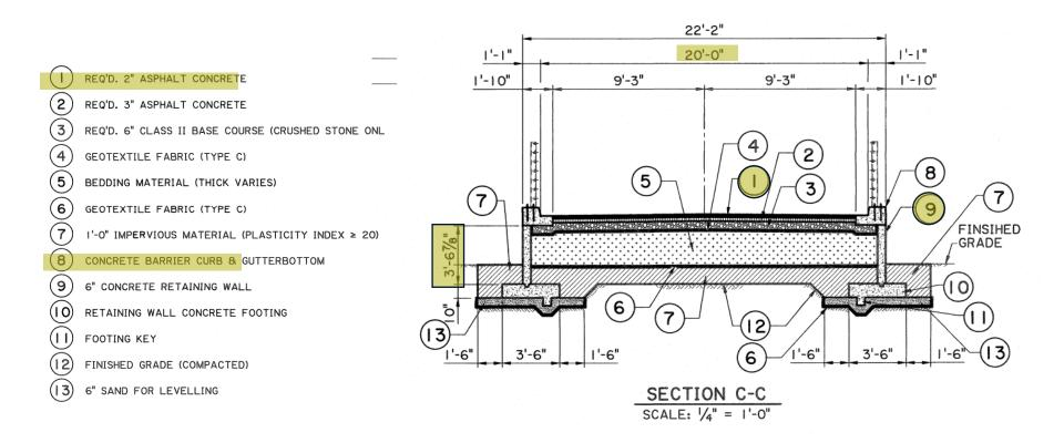
Ramp Approach Cross Section at Bridge (Conti Side)
